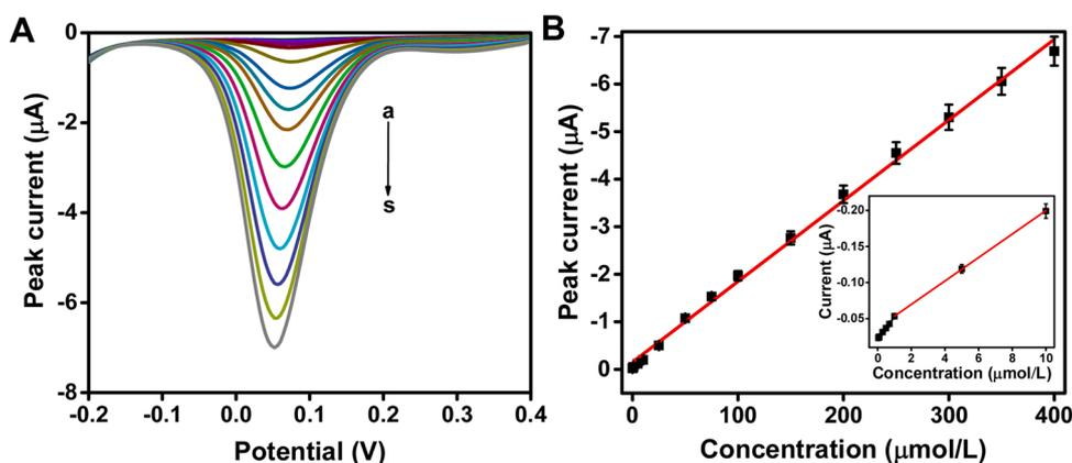
Fig. 8. (A) DPV curves at  $\text{Co}_3\text{O}_4@\text{TAPB-DMTP-COF}/\text{GCE}$  in  $0.1 \text{ mol} \cdot \text{L}^{-1}$  ABS with different concentrations of TBHQ (from a to s: 0.05, 0.07, 0.1, 0.3, 0.5, 0.7, 1.0, 5.0, 10, 25, 50, 75, 100, 150, 200, 250, 300, 350,  $400 \mu\text{mol} \cdot \text{L}^{-1}$ ). (B) The calibration curve of the reduction peak current vs. TBHQ concentration. Inset: the tendency of current intensity when TBHQ concentrations are low.
