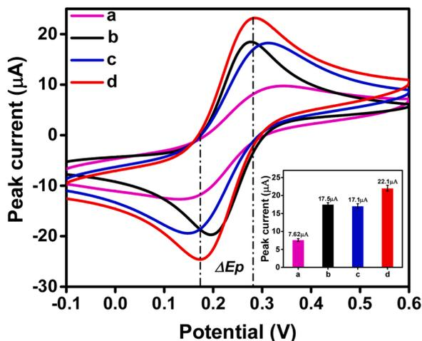
Fig. 4. CVs of  $0.5 \text{ mmol} \cdot \text{L}^{-1} [\text{Fe}(\text{CN})_6]^{3-/4-}$  containing  $0.1 \text{ mol} \cdot \text{L}^{-1} \text{ KCl}$  at bare GCE (a),  $\text{Co}_3\text{O}_4$ /GCE (b), TAPB-DMTP-COF/GCE (c) and  $\text{Co}_3\text{O}_4$ @TAPB-DMTP-COF/GCE (d). Scan rate:  $100 \text{ mV} \cdot \text{s}^{-1}$ .
