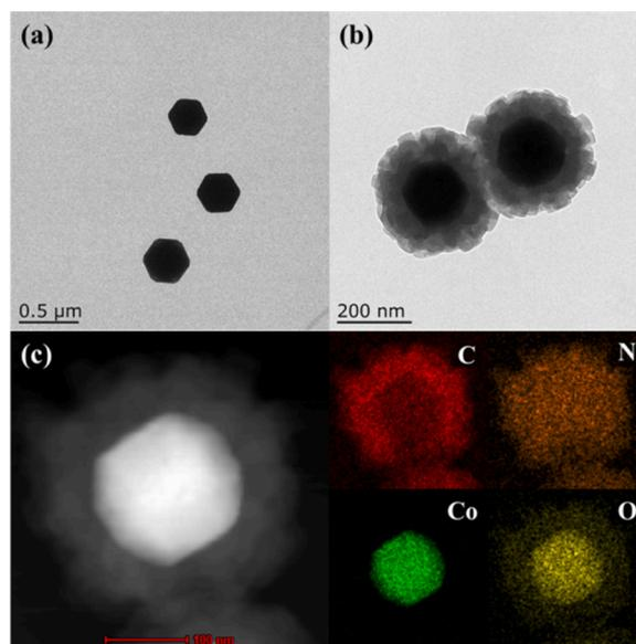
**Fig. 2.** TEM images of  $\text{Co}_3\text{O}_4$  (a) and  $\text{Co}_3\text{O}_4@TAPB-DMTP-COF$  composite (b). EDS-TEM elemental mapping (c) of C, N, Co, O for  $\text{Co}_3\text{O}_4@TAPB-DMTP-COF$  composite.
