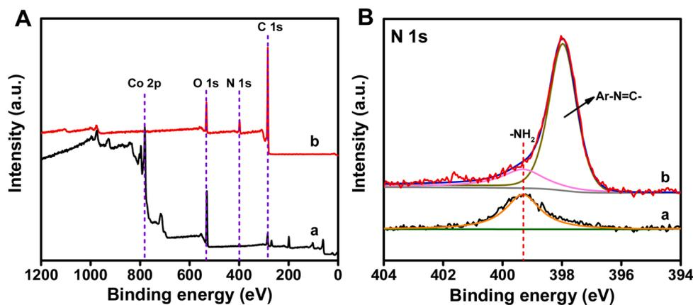
Fig. 3. (A) XPS survey spectra and (B) N 1s core-level XPS spectra of  $\text{Co}_3\text{O}_4$ -DMTP (a) and  $\text{Co}_3\text{O}_4$ @TAPB-DMTP-COF composite (b).
