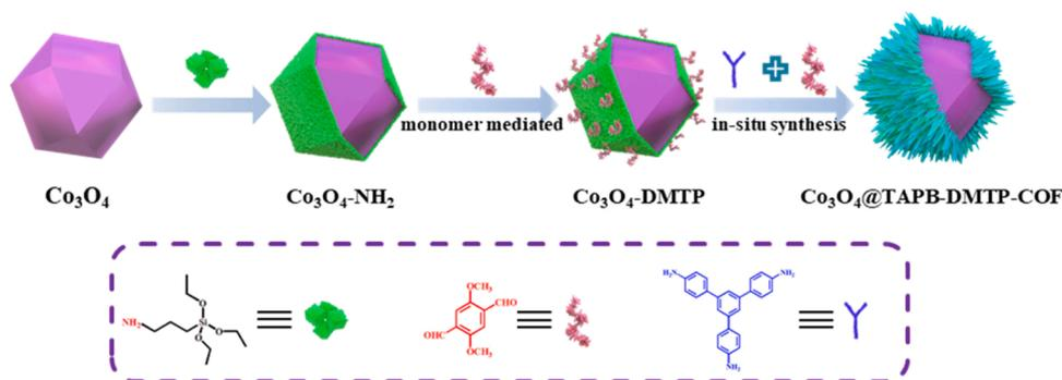
**Scheme 1.** Illustration of monomer-mediated in situ growth strategy for the synthesis of  $\text{Co}_3\text{O}_4@TAPB-DMTP-COF$  core-shell-structured composite.
