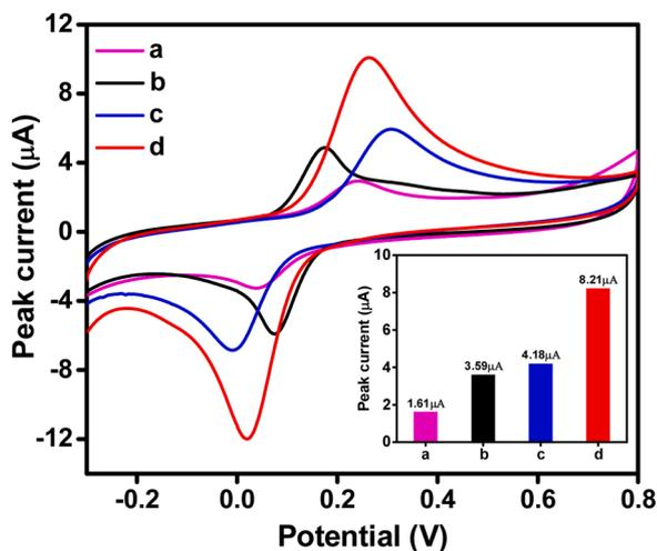
Fig. 5. Cyclic voltammograms obtained for  $100 \mu\text{mol L}^{-1}$  TBHQ at bare GCE (a),  $\text{Co}_3\text{O}_4/\text{GCE}$  (b), TAPB-DMTP-COF/GCE (c) and  $\text{Co}_3\text{O}_4@$ TAPB-DMTP-COF/GCE in  $0.1 \text{ mol} \cdot \text{L}^{-1}$  ABS (pH 5.0).
